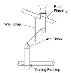
Figure 30 - Offset with Wall Strap and 45° **Elbows**
